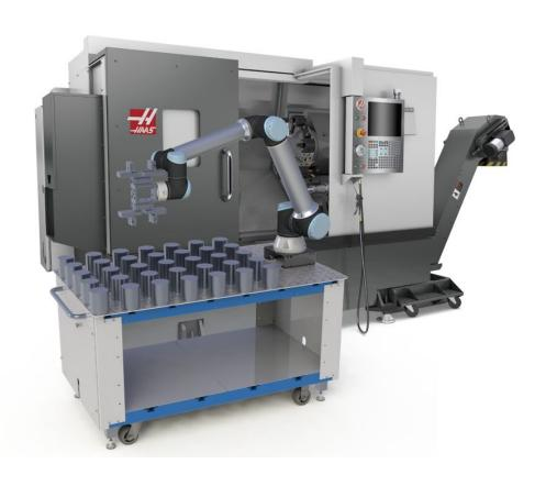
Thank you for purchasing the VersaBuilt Lathe Automation System. The Lathe Automation System is a tool for loading and unloading parts to your CNC lathe machine. Like many tools used in manufacturing, it requires training to use safely and effectively.
