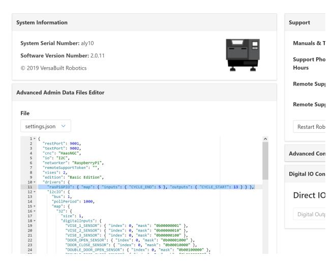
You will be editing line 11 (highlighted in this image). "CYCLE\_START": 13 should be changed to "CYCLE\_START": 19 for relay 2 or "CYCLE\_START": 16 for relay 3.
